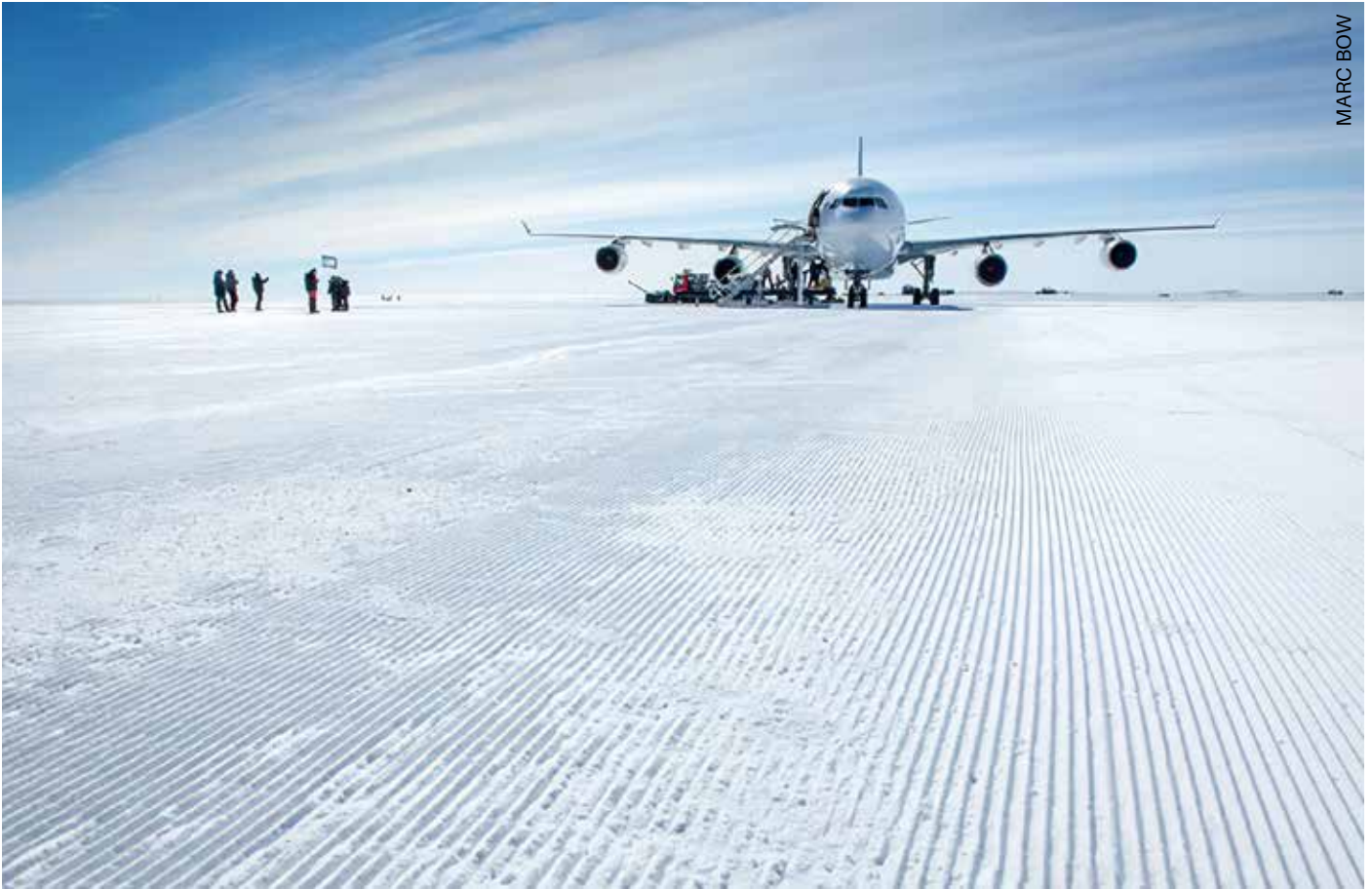
Picture of the first Airbus A340 landing in Antarctica. The grooves made on the ice to increase the grip are visible
