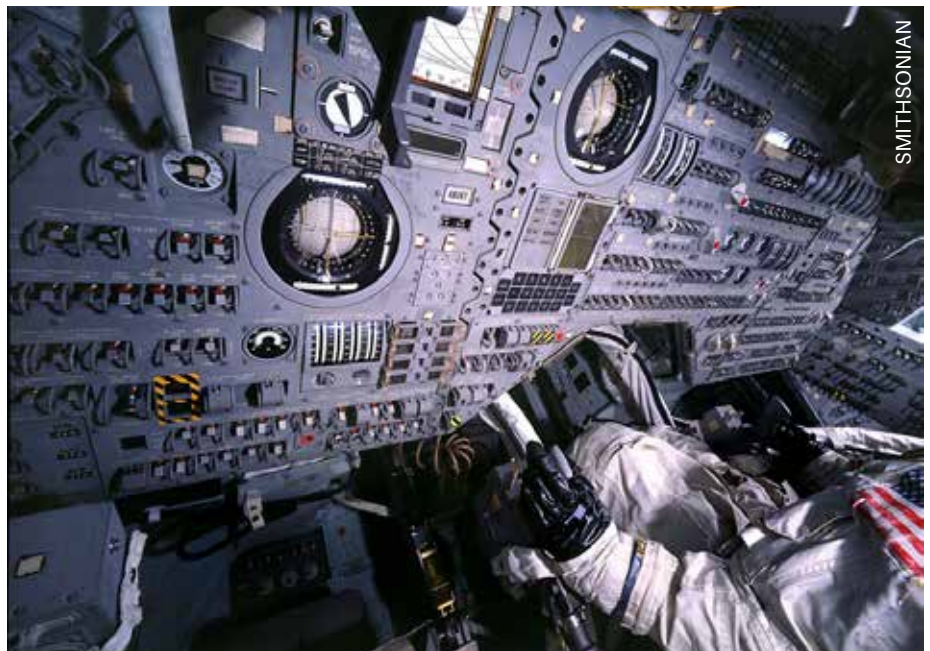
Figure 2: The view from the Commander's seat of the Apollo 11 Command Module Columbia
