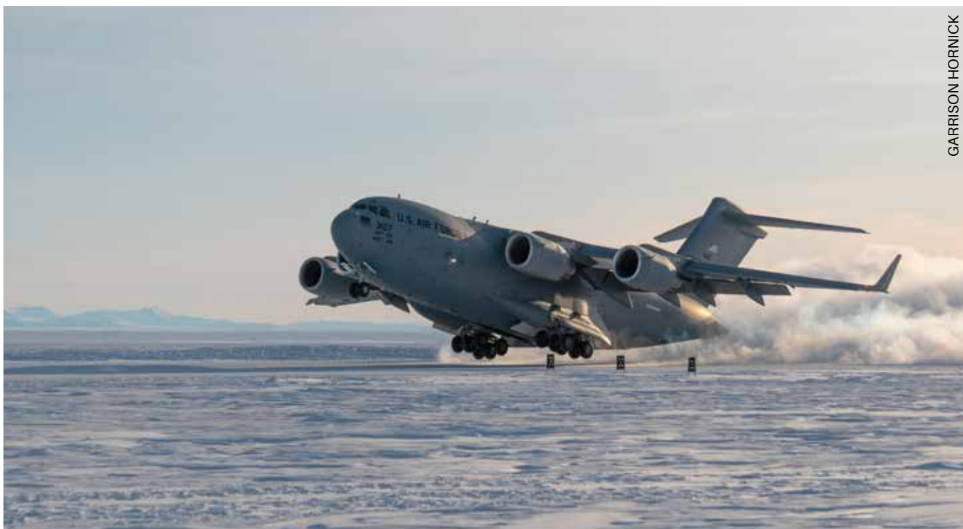
A Boeing C-17 Globemaster III taking-off at Antarctica. The markers make the end of the ice runway more visible
