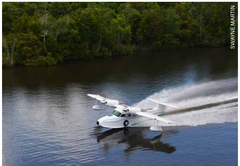
Amphibious flying boat performing a water landing. Despite landing on its fuselage, it also has floaters on its high wing in case of rough waters
