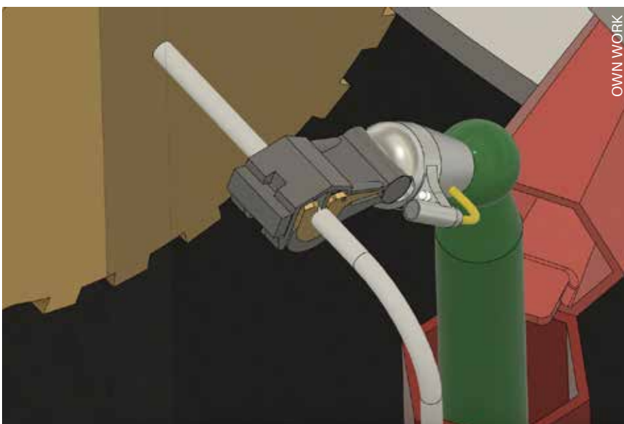
Figure 3: The endoscope out of the piercing tool, intercepting the wire
