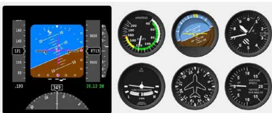
Figure 1: The same information shown on a Primary Flight Display (left) and analogue six-pack (right)
