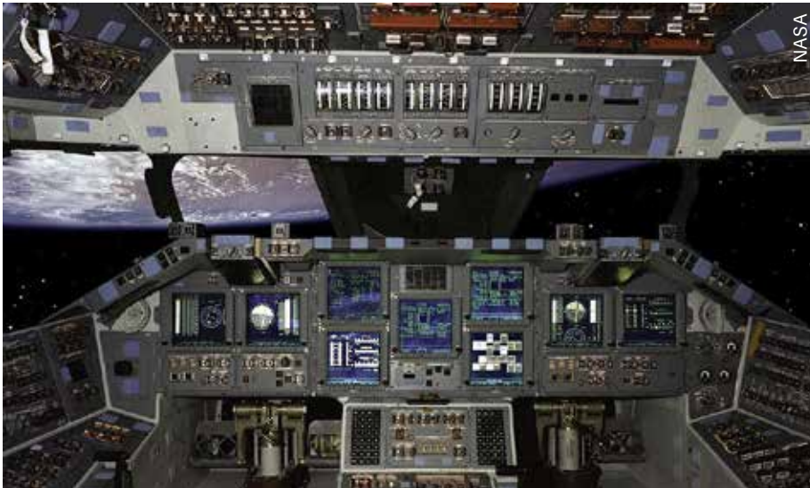
The upgraded glass cockpit. Note that this is a composite image from before the cockpit flew, as the seats have been removed!
