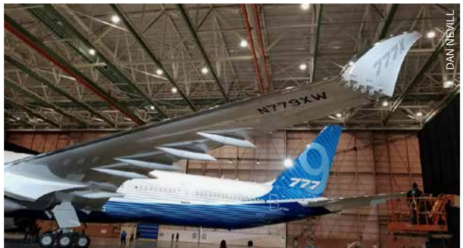
Figure 4: 777X Folding Wingtips
