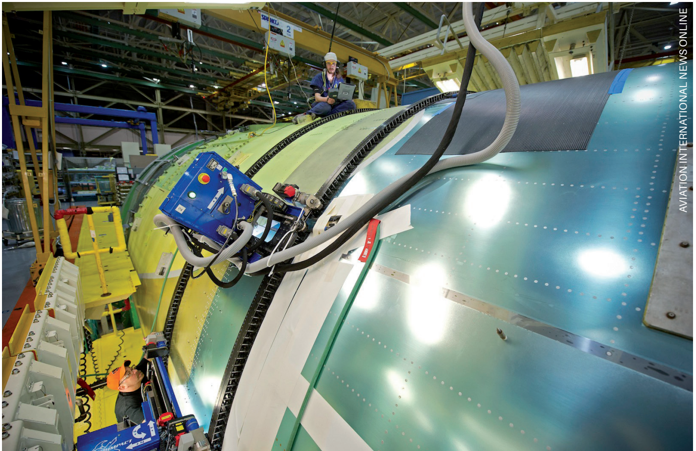
Figure 1: The Flex-Track system, mounted on the fuselage
