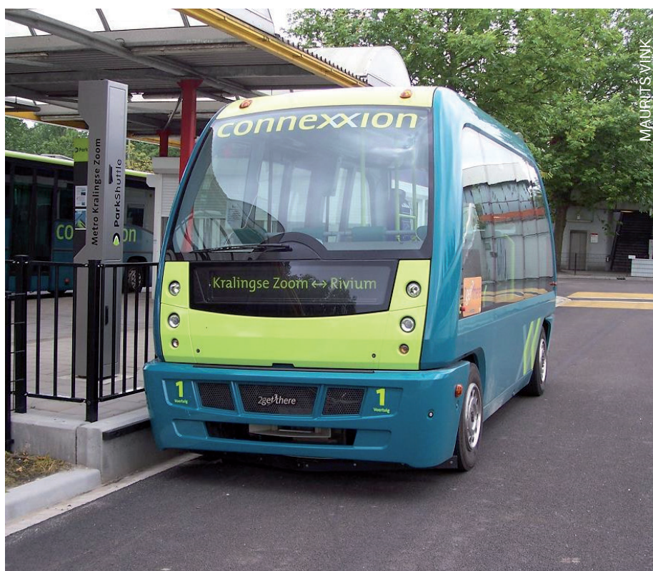
The ParkShuttle autonomous bus transports people between a few stops in the east of Rotterdam
