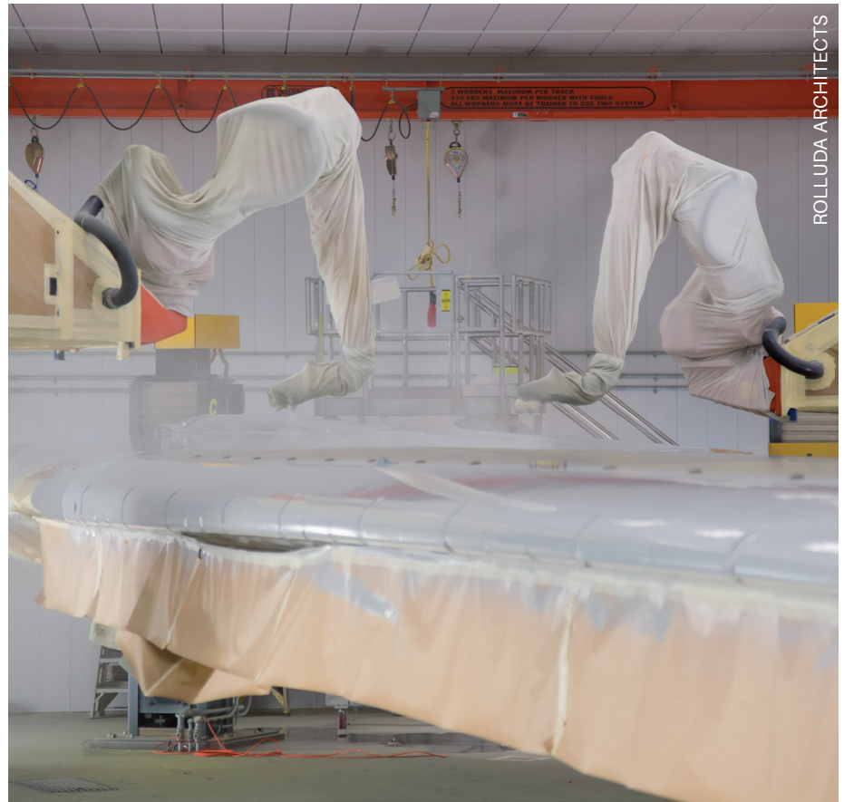
Figure 2: The Automatic Spray Method robots at work
