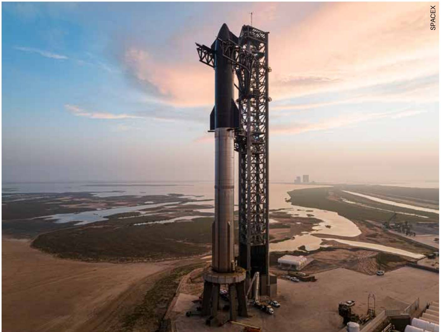
Starship fully stacked on its launchpad in Boca Chica, Texas. Black ceramic heat tiles for re-entry can be clearly seen covering the upper stage
