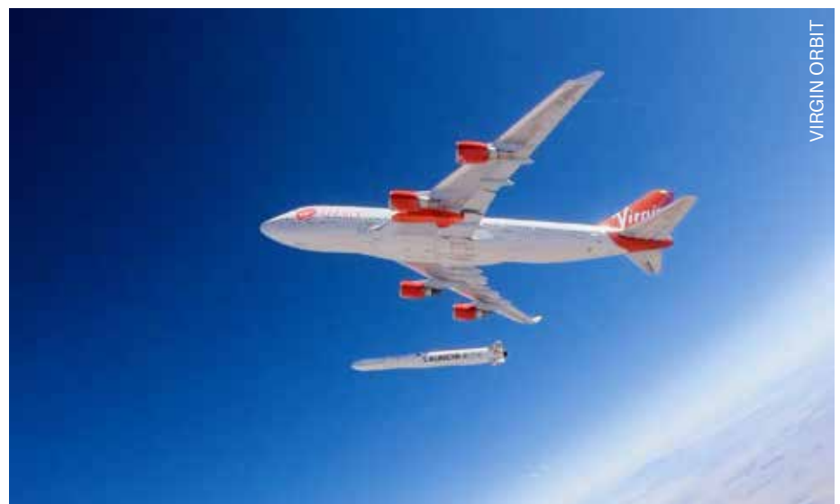
Virgin Orbit's Launcher One falling away from Cosmic Girl as part of a drop test
