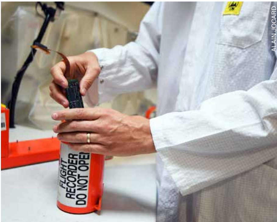
A Flight Data Recorder (FDR), one of the plane's black boxes, being opened for analysis
