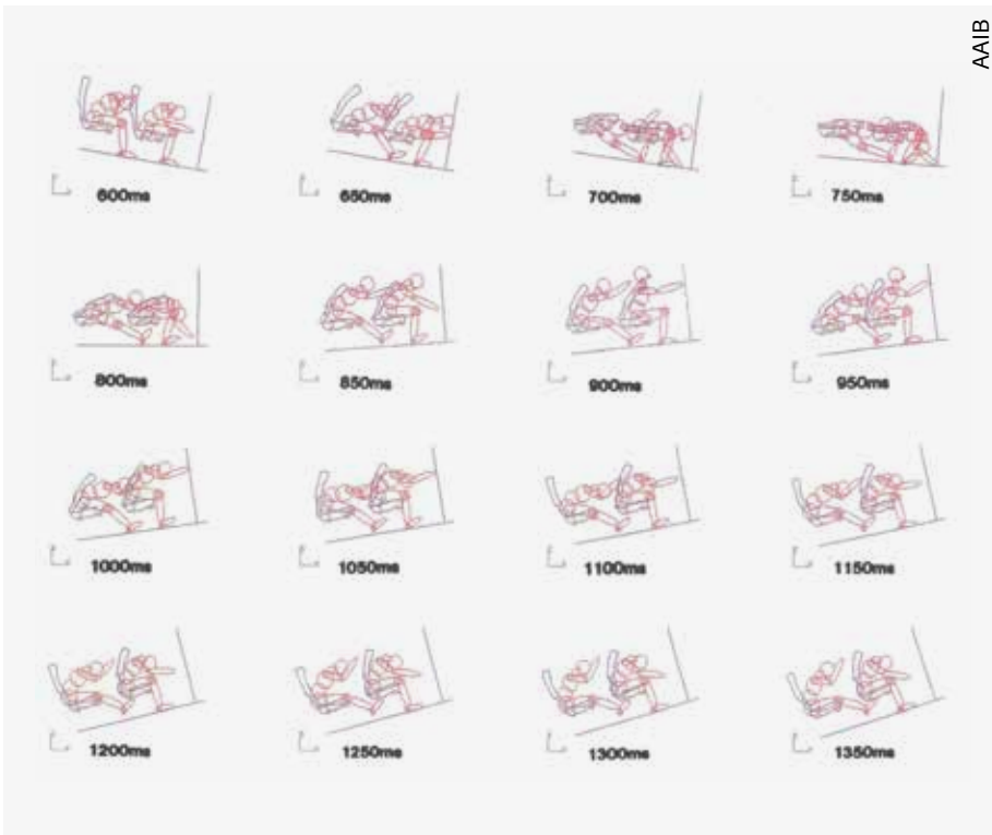
One of the simulations presented in the report after the Kegworth disaster displaying the dynamics of the brace position
