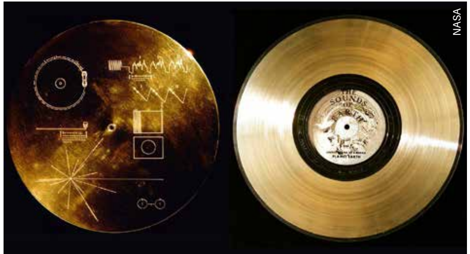
The Golden Record (right) and its protective cover (left), consisting of instructions to play the record, a pulsar map showing the location of our sun (lower left), and a depiction of the lowest state of a hydrogen atom (lower right)
