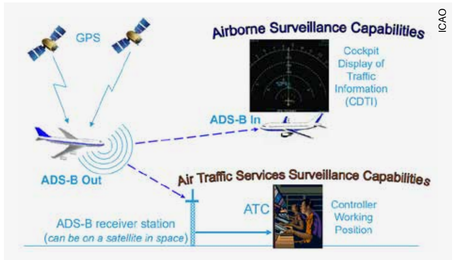
Aircraft calculate their position and transmit ADS-B Out signals. This is used by both Air Traffic Control and other aircraft, which receive ADS-B In and display traffic information to pilots
