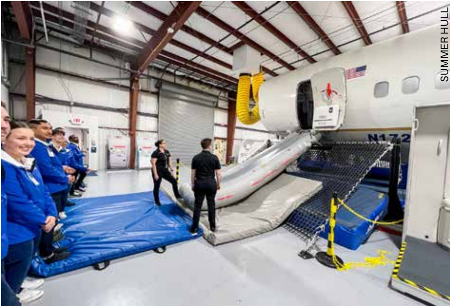
Flight attendants learning the deployment and use of the emergency landing evacuation slides
