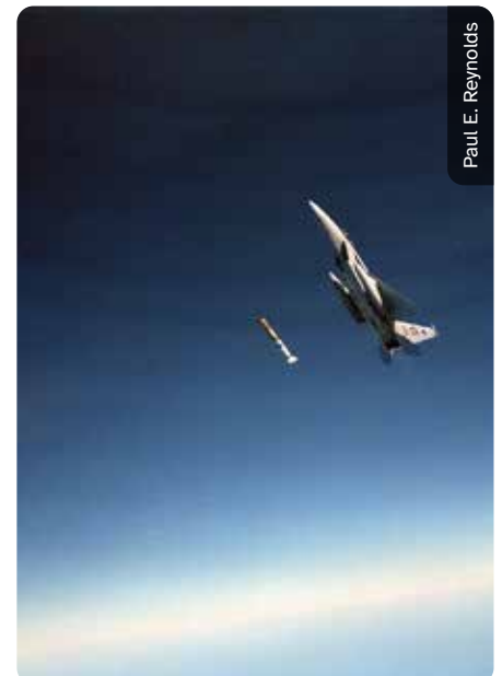
An F-15 releasing an ASAT during testing
