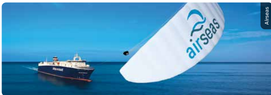
A kite made by Airseas used as auxiliary aid for the engines
