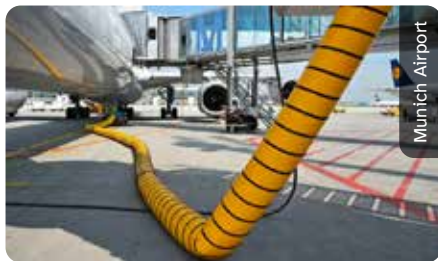
Figure 2: PCA unit in use at Munich Airport
