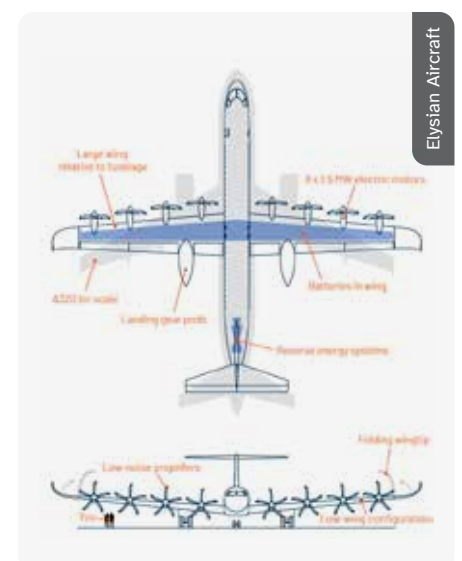
Engineering highlights of the E9X, with a reduced fuselage cross-section and an expanded wing span relative to the A320
